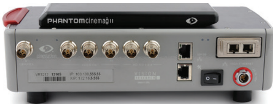
Phantom CineMag II installed on a Phantom CineStation-X2SR
