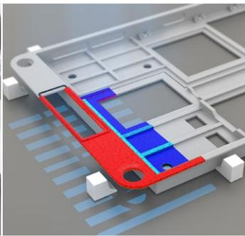
Gocator 3D snapshot sensors combine blue-LED structured light with built-in 3D measurement tools for high-precision area scanning and inspection. As opposed to lasers that are used to scan moving objects, snapshot sensors use a single snapshot scan to inspect stationary objects or objects with start/stop motion.
