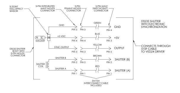
The synchronization system for DSS35B shutter devices incorporates a small magnet mounted to the driving mechanism and a Hall effect sensor. When the device achieves approximately 80% of full open, the magnet causes the Hall effect sensor to change state, producing a signal to indicate that the shutter has switched to the active state. Shown to the left is the DSS35B's shutter schematic which incorporates this electronic synchronization system.
