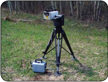
Figure 3: This long-range automated gas detection system scans large areas to detect gas leaks. In order to provide the required capability to geo-locate the gas leak, it is critical that the system be able to scan accurately in a "raster" pattern. Any error in pointing angle of that scan will result in erroneous geo-coordinates of the gas leak.
