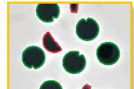
Detect contour defects.
