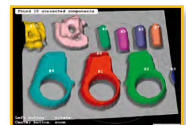
A 3D object model is segmented into connected components.
