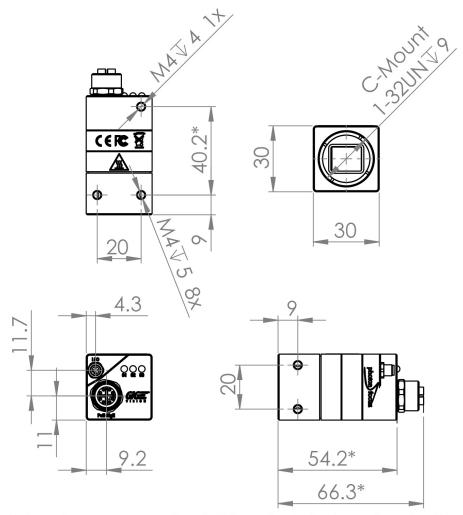
\*Dimensions may vary up to  $\pm$  0.8mm due to the type of construction
