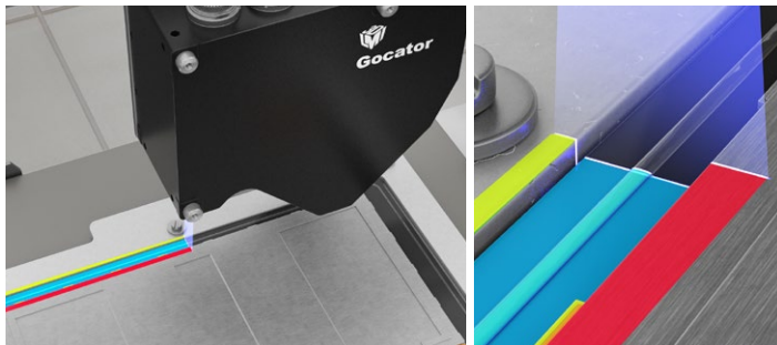
Transparent Glue Inspection with Gocator 2610
